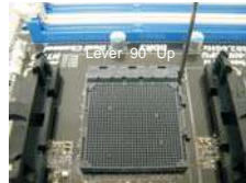
STEP 1: Lift Up The Socket Lever
