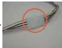
SATA power cable 1x4-pin power connector (White)
