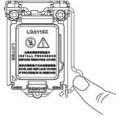
B. Lift the tail of the load lever and rotate the load plate to fully open position.
