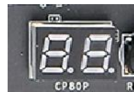
Debug LED with CPU Temperature Monitor
