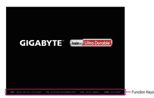
There are two different BIOS modes as follows and you can use the <F2> key to switch between the two modes. The Classic Setup mode provides detailed BIOS settings. You can press the arrow keys on your keyboard to move among the items and press <Enter> to accept or enter a sub-menu. Or you can use your mouse to select the item you want.
