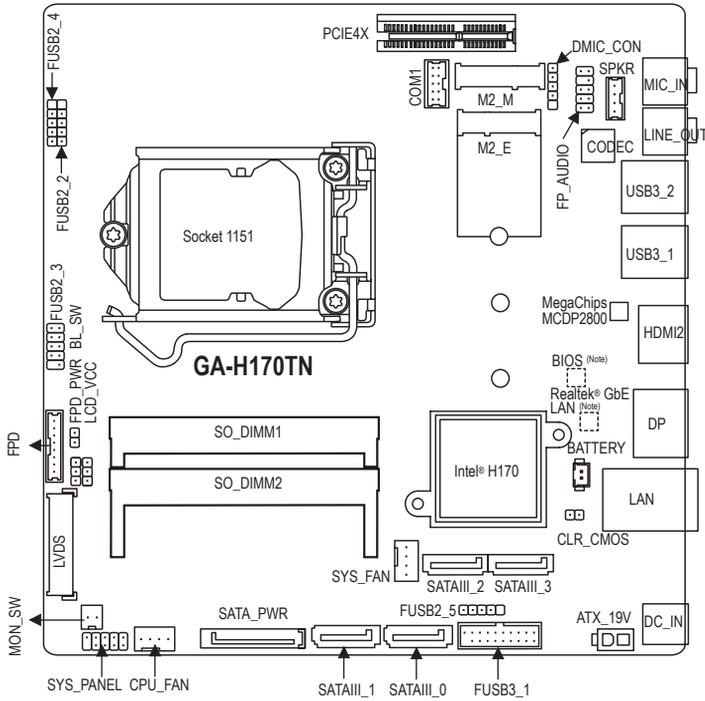
(Note) The chip is located on the back of the motherboard.
