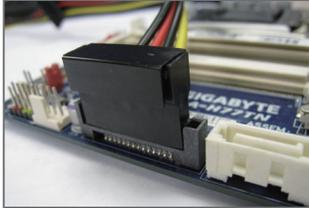
Connect the included SATA power cable to the SATA\_PWR connector. Then connect the SATA/optical drive power connectors to your hard drive and optical drive.
